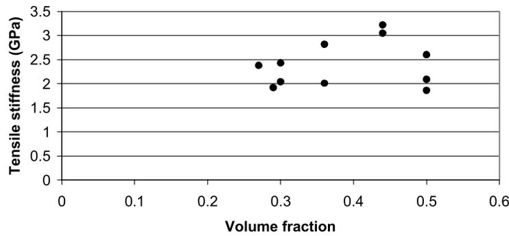
Fig. 6. The stiffness of tendon/glue composites plotted against tendon fibre volume fraction.
