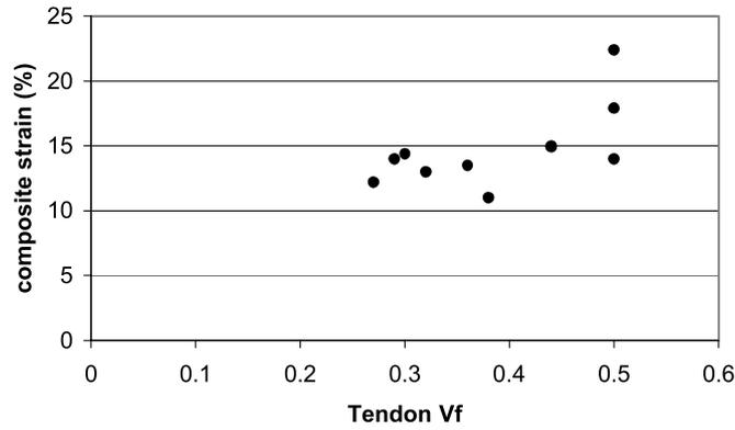
Fig. 8. The failure strain of tendon/glue composites plotted against tendon fibre volume fraction.
