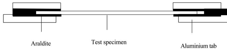
Fig. 1. Diagram showing the metal tabs that were glued onto the ends of the tensile specimens to prevent the ends being crushed during clamping.
