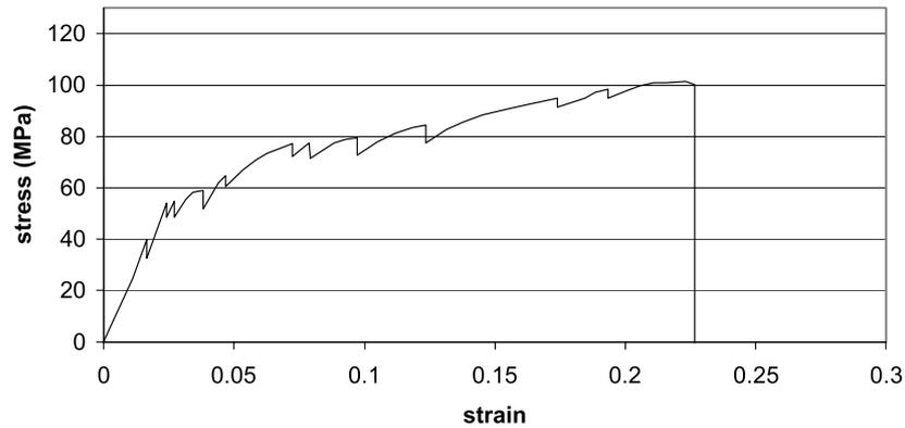
Fig. 4. A typical stress/strain curve for dry composite at a volume fraction of 50%, tested in tension.
