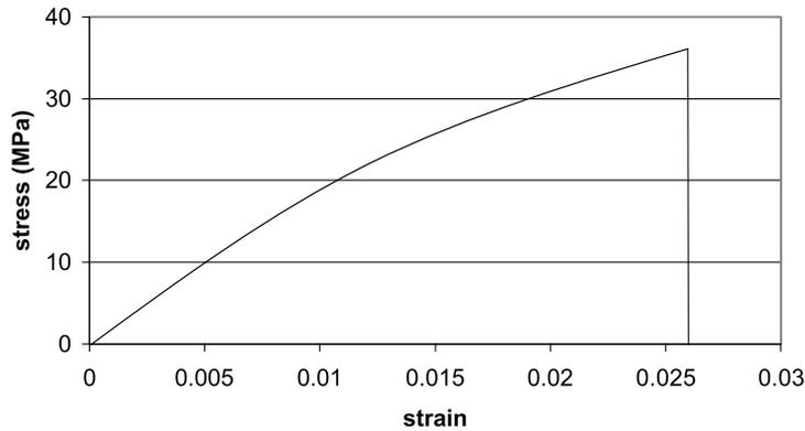
Fig. 2. A typical stress/strain curve for dry pearl glue tested in tension.
