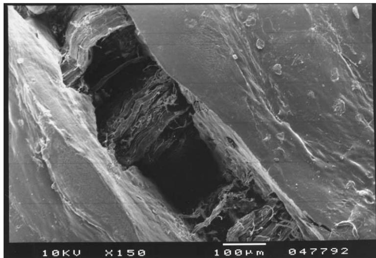
Fig. 5. An electron micrograph showing a crack in tendon/glue composite deformed to a strain of 18%. Collagen fibres can be seen bridging the crack and the crack has not closed up after removal of the load, indicating that irreversible deformation has occurred.
