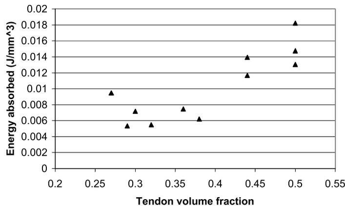
Fig. 9. The energy absorbed to failure by tendon/glue composites plotted against tendon fibre volume fraction.
