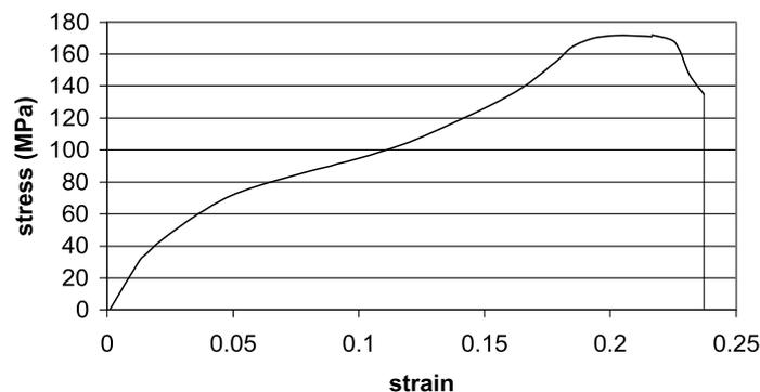
Fig. 3. A typical stress/strain curve for dry whole tendon tested in tension.
