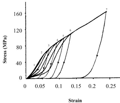
Fig. 10. Stress strain curve for a whole dry tendon repeatedly loaded and unloaded in tension. The numbers show the magnitude to which successive loads were applied and the direction of unloading is indicated by arrows.
