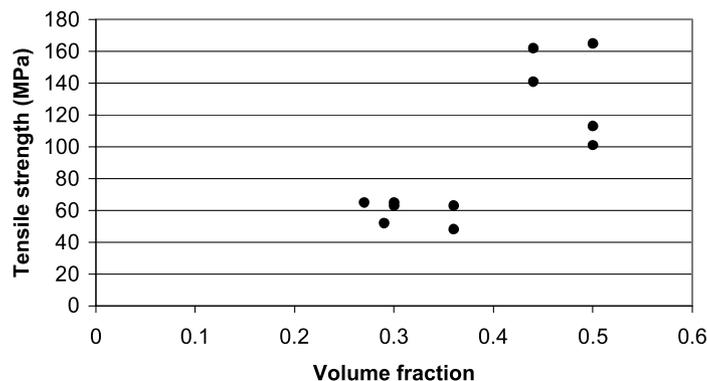
Fig. 7. The strength of tendon/glue composites plotted against tendon fibre volume fraction.
